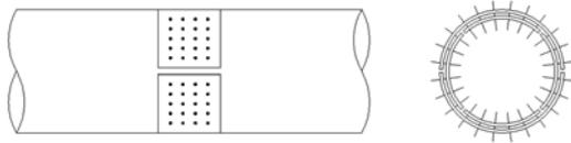
**Fig.C10.6.6 Example of 4-way splitting of a restrainer plate**
