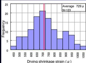
According to JIS test, the average shrinkage strain of concrete is 730 μ .
