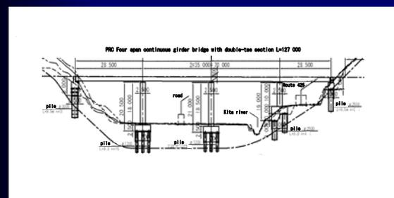
(Adopted Plan) 4-span continuous PRC double girder bridge
