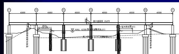
(Adopted plan) 6-span PC simple girder bridge 40m × 6=240 m.
