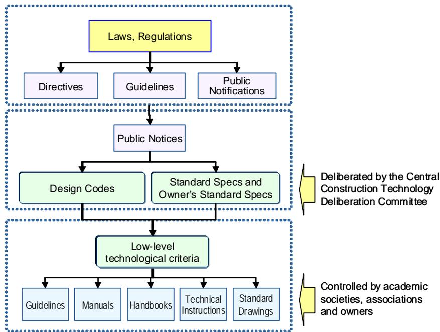
Figure 1. Design codes and standard specifications in Korea
