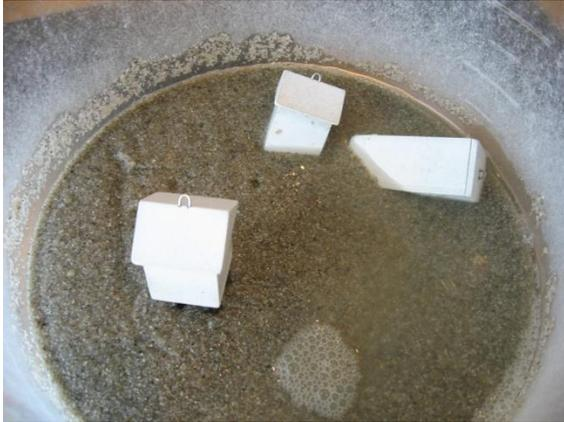
**The model house at the bottom left has pile foundation. Liquefaction has minimal effect on it.**
