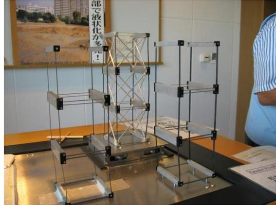
**The cross-braces and base isolators reduce the effect of Earthquake on high rise buildings.**
