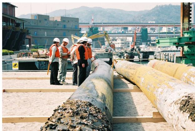
Fig. 4 Damage to steel piles for pile-supported-wharf in Kobe Port during 1995 Hyogoken-Nambu earthquake
